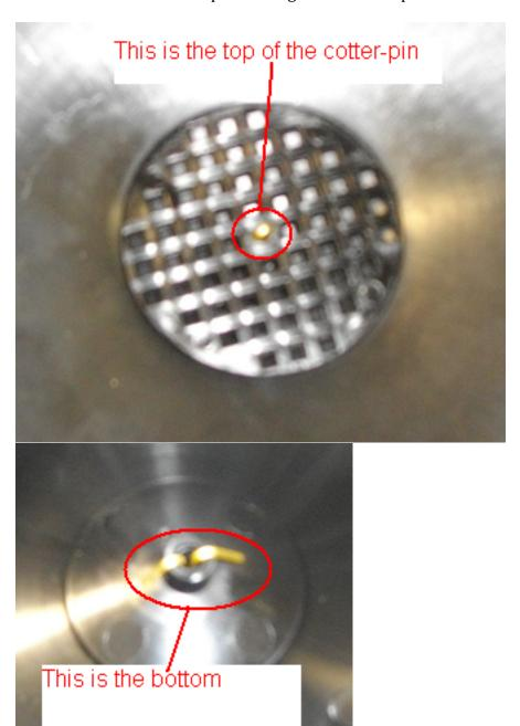
• Remove the cotter pin by bending the legs at the bottom back straight and pushing it back towards the top of the collector. Once the cotter pin is removed you can pop out the screen. You may need a small tool such as a knife to help pop the screen out. Once the screen is removed you will be able to see the drain hole.
