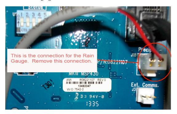
• Once the wire has been removed, you will see two gold legs. Use a screwdriver to short out these two pins. Make sure the screwdriver is touching both pins at the same time, multiple times. If this results in rainfall counts, there is an issue with the wire going to the rain gauge, the connection from that wire to the reed switch is not well connected, or the reed switch is faulty. Should this not result in rainfall data, there is an issue with the motherboard.
