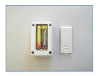
Install the two AAA batteries supplied. The green LED will flash rapidly as the RainLog powers up.
