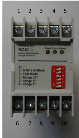
Figure 1: The front of the device, showing the terminal numbers labeled.
