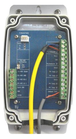
When replacing the cover, make sure that all installed cables are pinched by the black foam on the bottom of the enclosure. This will enable a weather tight seal.
