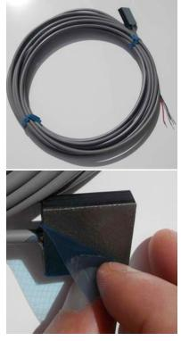
If the cable length of 25ft. is insufficient for the installation, additional cable can be added to the existing cable. If this is done, an accuracy-derating factor must be added to the overall temperature accuracy of this sensor. For every 100ft. of cable added, a derating factor of -0.125C must be taken into account.
